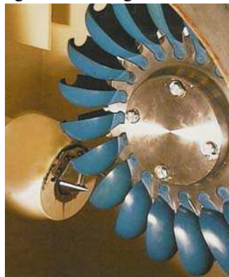
Figure 3.1.3.2. Pelton blades of plastic
